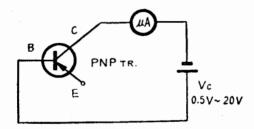
It can be measured if one is provided with a microampere meter and a battery. Ico value has little to do with the size of Vc, while it is affected more by temperature. If, however, Vc is in excess of a certain voltage, Ico will suddenly increase. The voltage on the bend of the increase curve is known by gradually raising Vc by way of a voltmeter connected in series.
