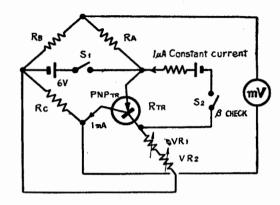
VR2 (0 adjustment) and to the base is given 1 microampere constant current. The impedance of the transistor ( $R_{TR}$ ) decreases and Ico increases in proportion to the  $\beta$  value, resulting in so much voltage drop by Rc. This unbalanced voltage of the bridge is measured on a highly sensitive millivolt meter to obtain the value on the scale converted to  $\beta$  value.
